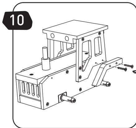
**EN** Attach part (F) to part (G) with screws (S1). Do the same on the other side.
