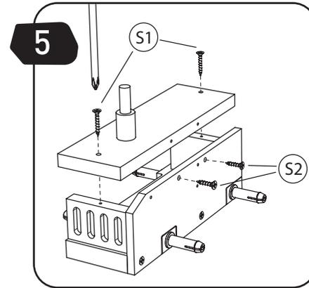
**EN** Attach part (E) to parts (A, B, D) with screws (S1, S2).
