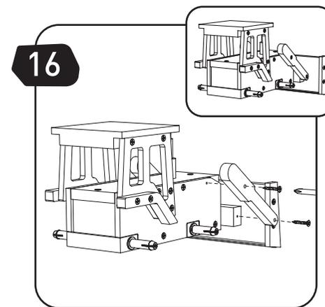
**EN** Attach part (K) to parts (A) and (L) with screws (S1).
