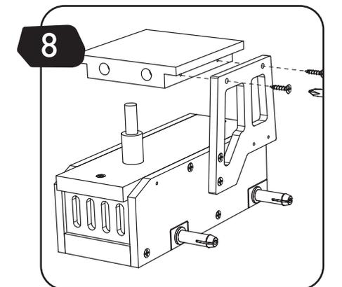
**EN** Attach part (H) to part (G) with screws (S2).
