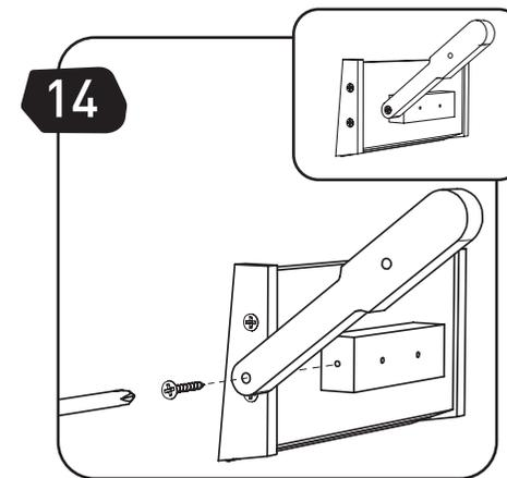
**EN** Attach part (K) to part (L) with a screw (S1).
