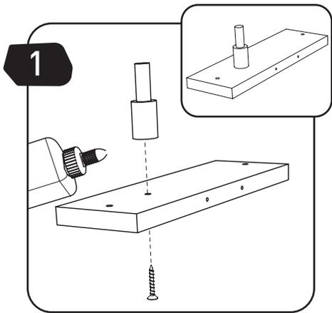
**EN** Apply glue to part (N) and attach to part (E) with a screw (S1).
