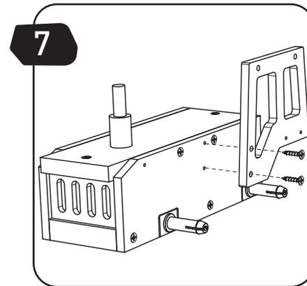
**EN** Attach part (G) to part (A) with screws (S2).
