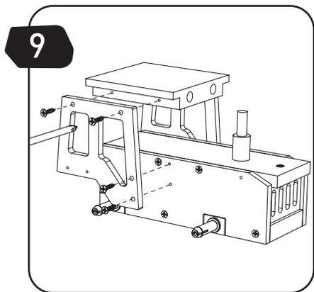
**EN** Attach part (G) to parts (A) and (H) with screws (S2).
