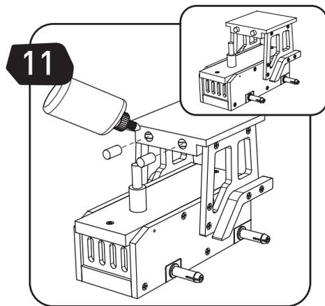
**EN** Apply glue to the holes in part (H) and attach parts (O).
