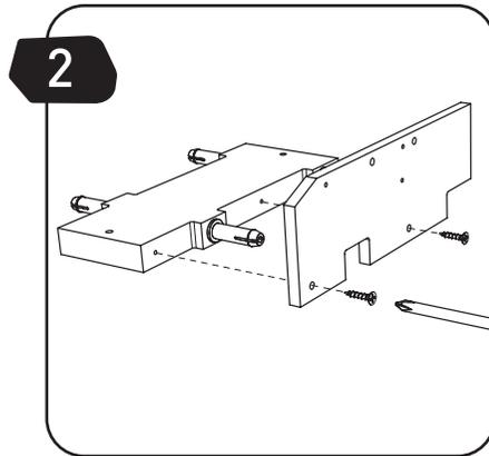
**EN** Attach part (A) to part (C) with screws (S2).
