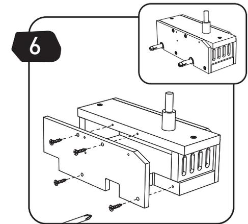
**EN** Attach part (A) to parts (E,C) with screws (S2).
