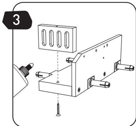
**EN** Apply glue to part (B) and attach to part (C) with a screw (S1).
