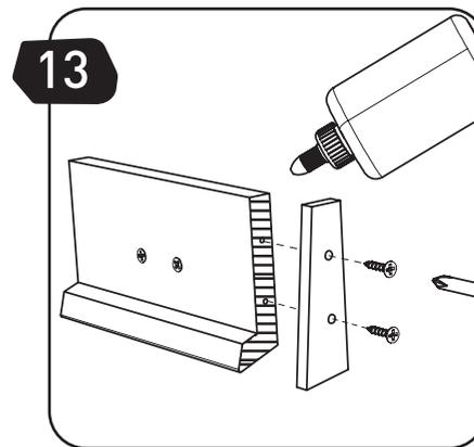
**EN** Apply glue to part (J) and attach part (M) with screws (S2). Do the same on the other side.
