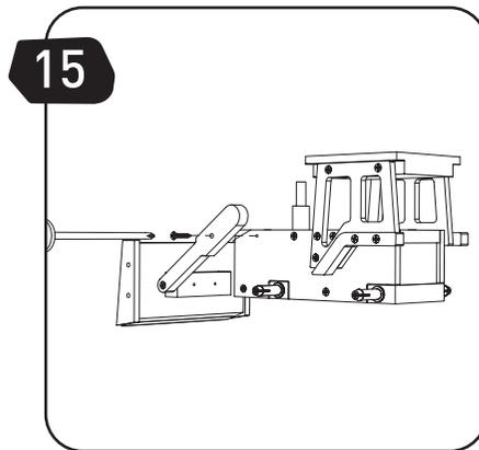
**EN** Attach part (K) to part (A) with a screw (S1).
