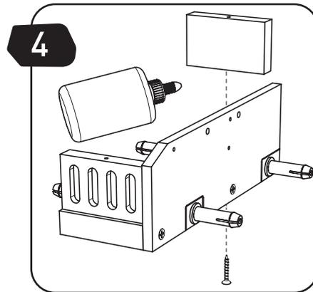
**EN** Apply glue to part (D) and attach to part (C) with a screw (S1).
