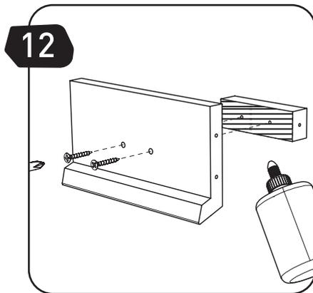
**EN** Apply glue to part (L) and attach to part (J) with screws (S1).
