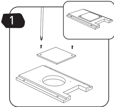
**EN** Attach part (F) to part (A) with screws (S3). Repeat this step with the two identical parts.
