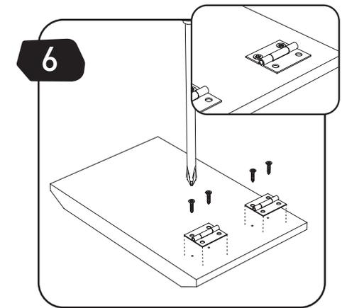
**EN** Attach the hinges to part (D) with screws (S3).
