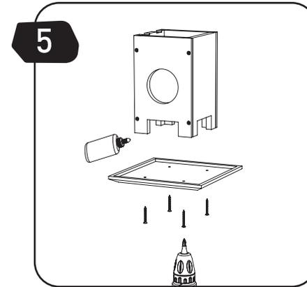
**EN** Apply glue to the bottom of the assembled part, and attach part (E) with screws (S1).
