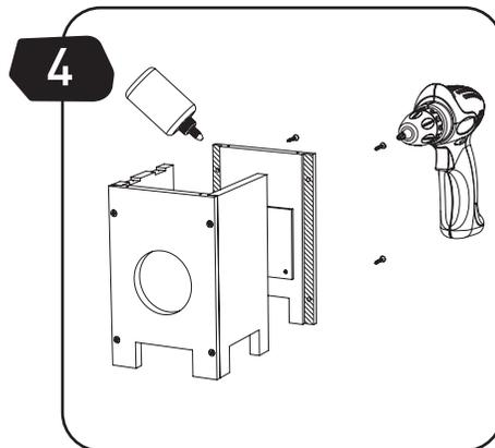
**EN** Apply glue to the sides of part (A) and attach to parts (B) and (C) with screws (S2).
