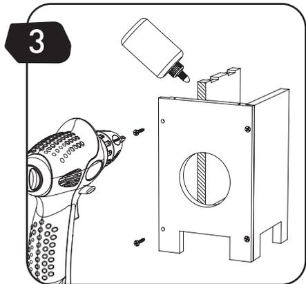
**EN** Apply glue to the side of part (C) and attach to part (A) with screws (S2).
