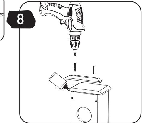
**EN** Apply glue to the side of part (A) and attach part (G) with screws (S1).
