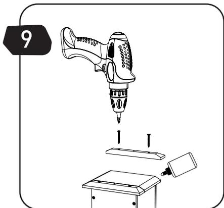
**EN** Apply glue to the side of part (A) and attach part (G) with screws (S1).
