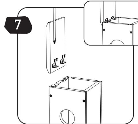
**EN** Attach the hinges (I) along with part (D) to part (C) with screws (S3). Close the cover.
