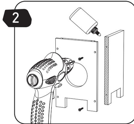
**EN** Apply glue to the side of part (B) and attach to part (A) with screws (S2).
