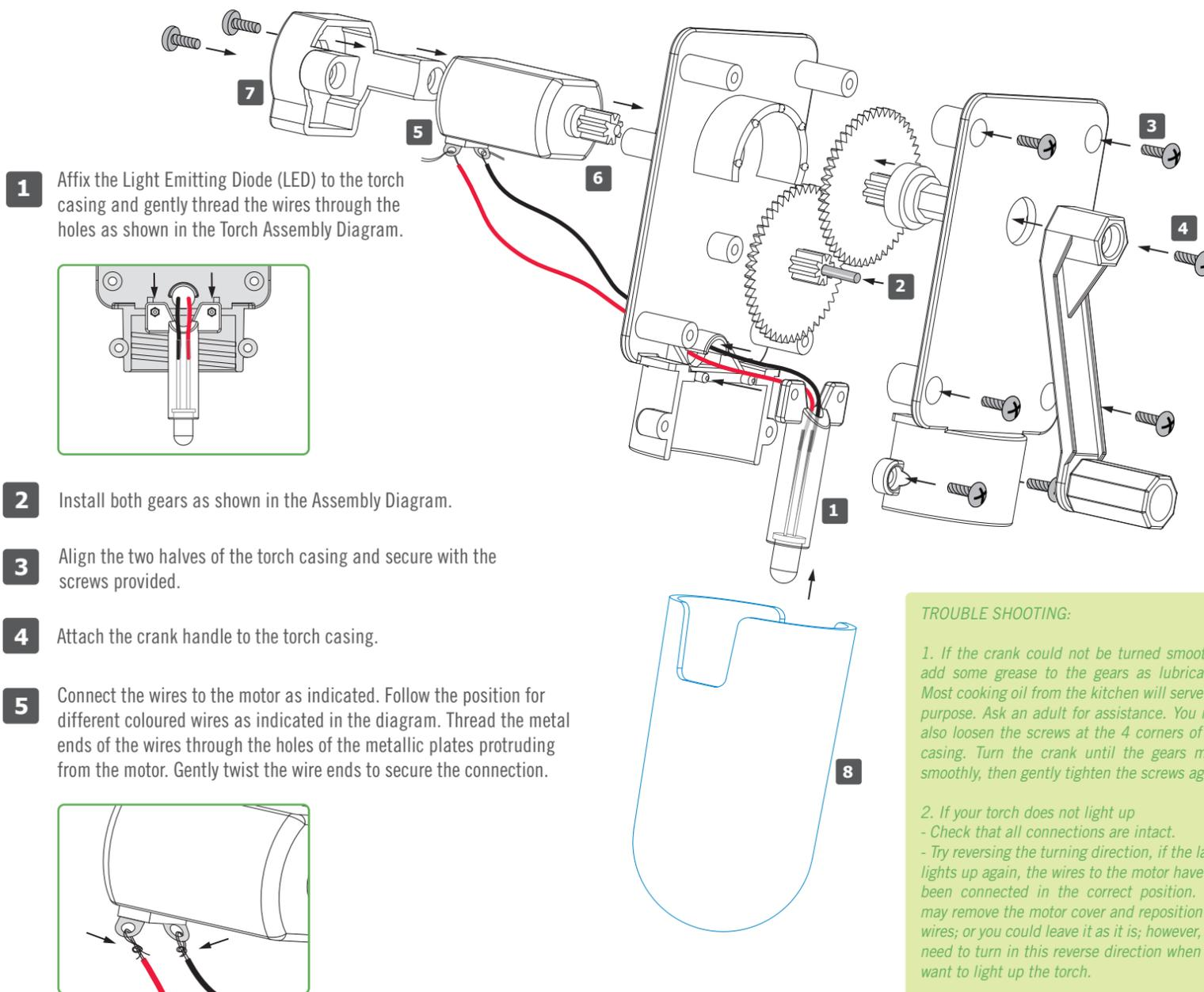
**1** Affix the Light Emitting Diode (LED) to the torch casing and gently thread the wires through the holes as shown in the Torch Assembly Diagram.
