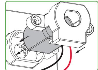
**7** Using 2 screws, secure the motor by aligning the cover to the base.
